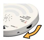
To adjust the volume, turn the thumbwheel up or down.
